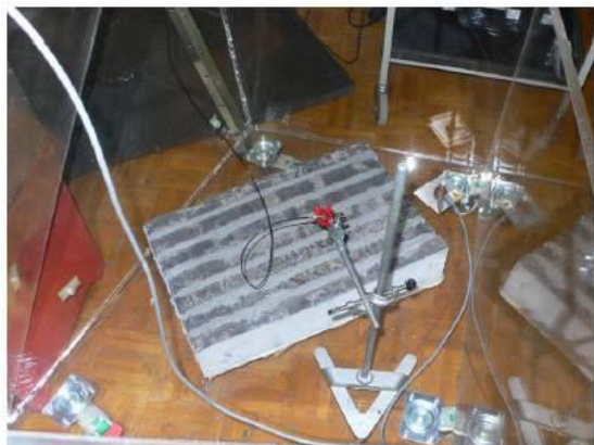
Fig. 4: Brick sample in the (transparent) model Reverberation chamber.
